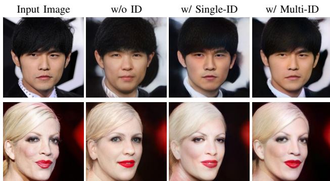
Fig. 6. The effect of multi-layer identity loss. With the multi-layer identity loss, the identity consistency between the reconstructed image and the input image is significantly improved.
